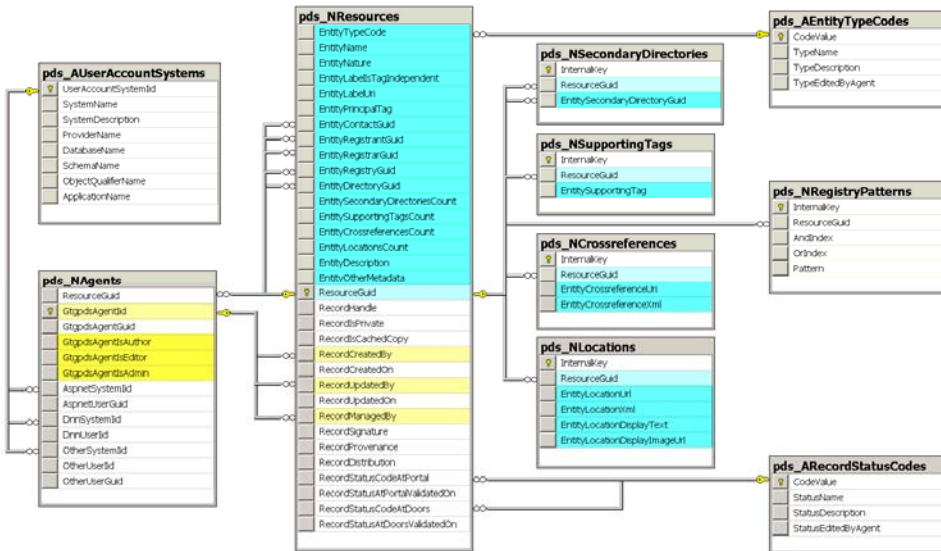
Fig. 3. Relational database model for NEXUS combined design server with integrated storage of both PORTAL and DOORS data record fields.
